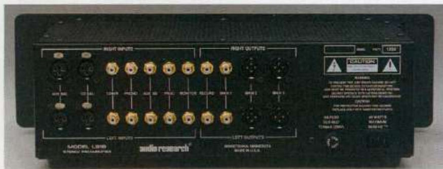
➤ Rear socketry array includes balanced and single-ended inputs and outputs
